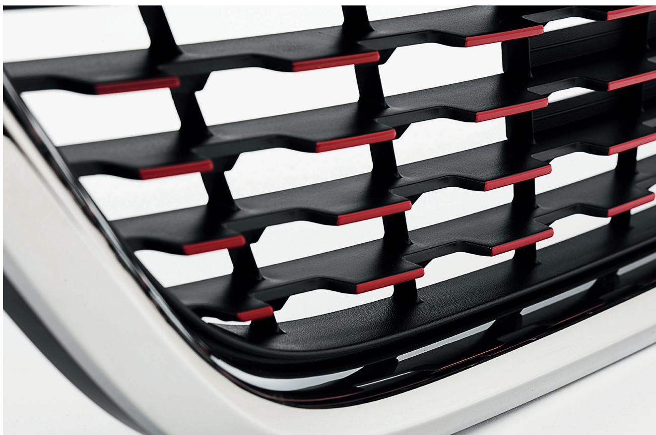
The radiator grille of the Peugeot 208 is hot-stamped from Luran S778T acrylonitrile styrene acrylic ester (ASA). The material is pre-colored, unpainted and suitable for long-lasting outdoor applications (© Ineos Styrolution)
